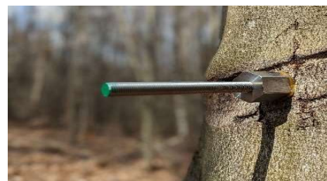
2.3.8 Screw in the wooden platform holder with inox guard ratchet
