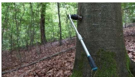
2.3.7 Screw the bolt into the end position using the telescopic
