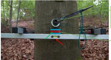
Attach the drilling device. Use the **spirit level** to align and tighten with nut and washer.
