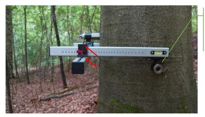
Loosen the clamping screws and shift the first arm to the desired position.
