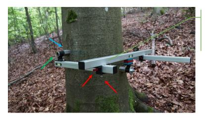
Untighten the clamping screws and align the drill sleeve with the platform screw.
