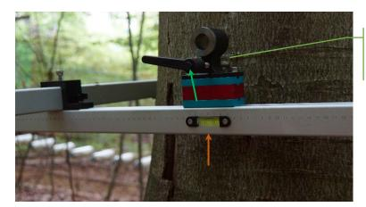
Attach the 4th arm to the trunk using the centring unit.
