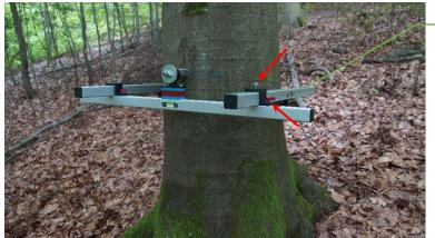
Loosen the **clamping screws** and shift the first arm to the desired position.
