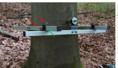
Untighten the clamping screws and shift the second arm to the desired position by using the scale.
