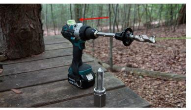
A multi-stage hole is now drilled in accordance with the installation instructions for platform bolts using a battery-powered screwdriver with spirit level or a drilling device.
