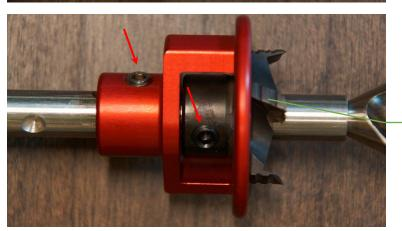
Determine the position of the countersink and the depth stop in accordance with the screw type.
