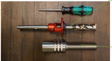
IMPORTANT: Before tightening the two Allen screws, align the surface of the drill shaft (hexagon) perpendicular to the two Allen screws.
