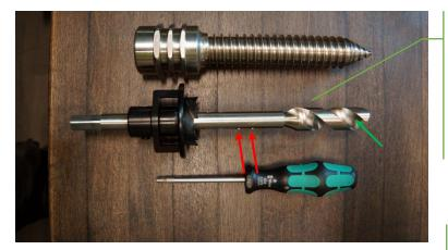
Select the drill diameter that matches the screw.
