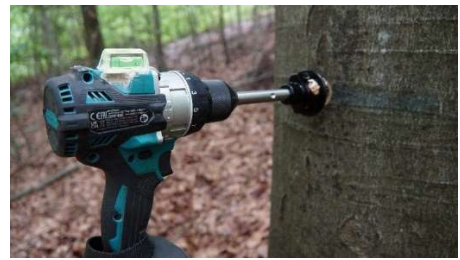
2.3.2 Drill the hole to the desired depth.
