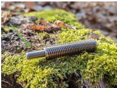
2.6.5 In softwood, installation with RAMPA socket type SKL, stainless steel 1.4305, D 18.5, d M10, L 80 mm is recommended as an option. ETA-12/048 1
