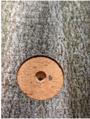
2.6.1 Create a flat surface with a \varnothing 40 mm forest drill.
