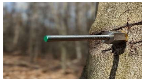
2.3.8 Screw in the threaded rod with inox guard
