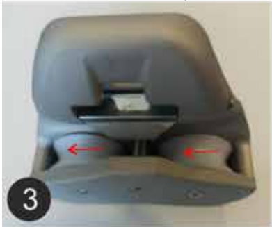
2 Checking of MCD wear (Free space between Locking Part and Plate 7,5 < x < 8,7\text{mm} )
