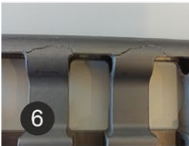
6 Check that IMN & CLiC-IT CBS anchorages have not suffered deformations due to shocks, deformations due to overstress in the screw housings or in the hole where the safety cable passes.
