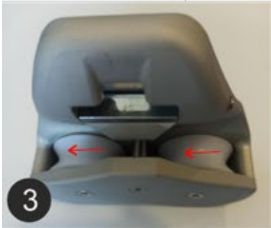
2 Checking of MCD wear (Free space between Locking Part and Plate 7,5 < x < 8,7\text{mm} )
