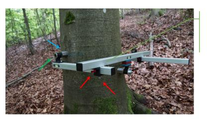
Untighten the clamping screws and align the drill sleeve with the BABO BOLT
