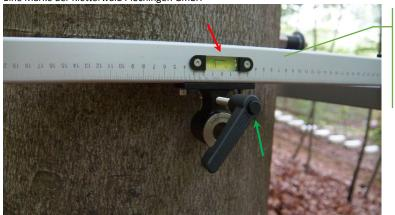
Align the lateral arms using the **spirit levels** and fix them to the trunk by using the **centring units**.
