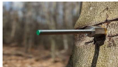
2.3.8 Screw in the threaded rod with inox guard
