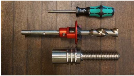
2.3.1 Set the multi-drill tool to the screw.
