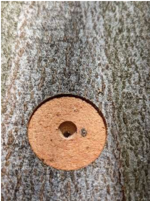
2.6.1 Create a flat surface using the 40mm diameter positioner drill bit
