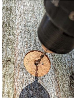
2.6.2 Prepare a 4 cm deep hole with a 4 mm drill bit.
