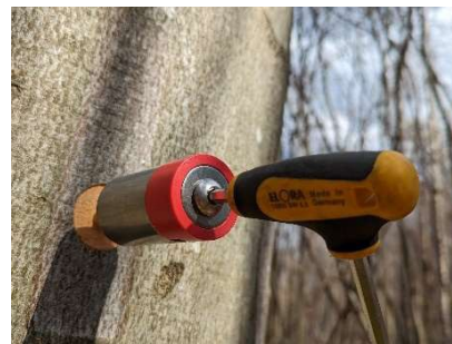
2.6.4 Screw in cable carrier with SW6 Allen key.
