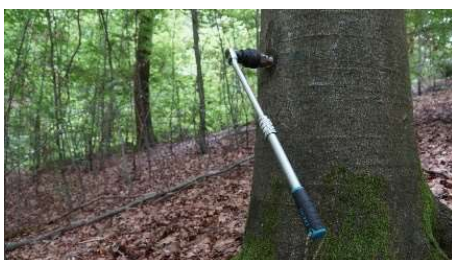
2.3.7 Screw the BABO BOLT into the end position using the telescopic ratchet.
